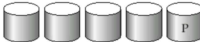
(e) RAID 4: block-interleaved parity
